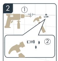
1- Drill holes (Ø 10 mm) into the spots you have marked. 2- Nail the wall plugs (D) in the holes by using a hammer.
