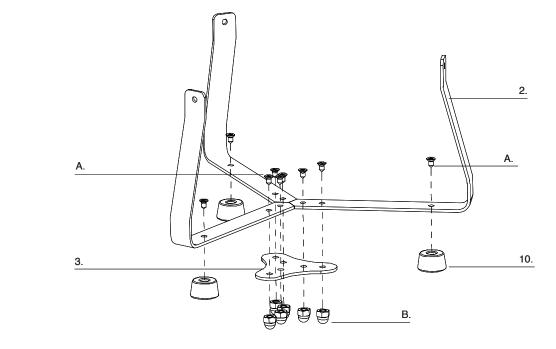
**STEP 1** - Secure the 3x bracket(2) & Triangle connection piece(3) to using the 6x screws(A) with the 6x dome-headed nuts(B) and using the 3x screws(A) with the 3x rubber stopper(10).
