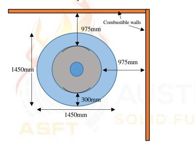
Figure 1 – Clearance Diagram
